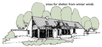
larger window openings on the sunny (south) side with shading to control summer daytime solar gain
